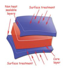
**FXPB** BOPP film with outstanding transparency and brilliance, both sides treated, non heat sealable, very good tensile strength and low elongation.
